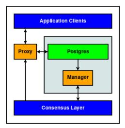
The consensus layer is an external entity where HARP Manager maintains information it learns about its assigned Postgres node, and HARP Proxy translates this information to a valid Postgres node target. Because HARP Proxy obtains the node target from the consensus layer, several such instances can exist independently.
