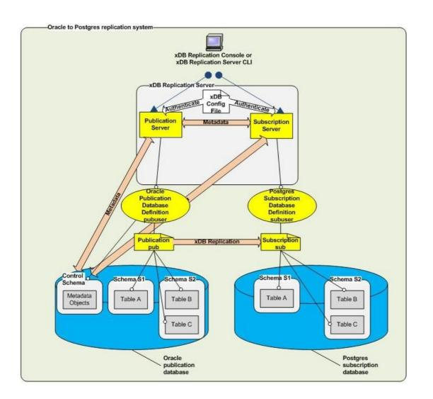
The following describes the logical components in the preceding diagram: \* The publication server to use is identified by registering its network location, user name, and password.
